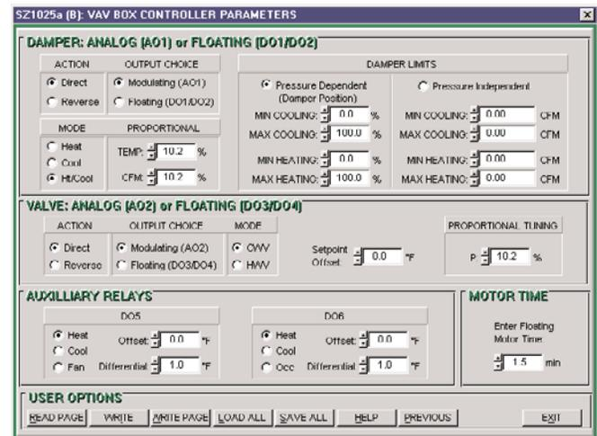
Select one of the following three models for the damper output: “Heat” mode, “Cool” mode and “Heat and Cool” mode which requires a supply air sensor.
