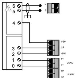
Optional QE25 Tri-state Interface Wiring
