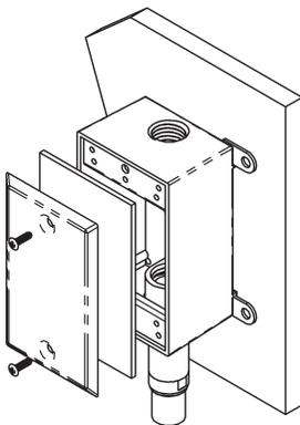
**Fig. 4:** Outside Humidity in a Weatherproof (WP) Enclosure
