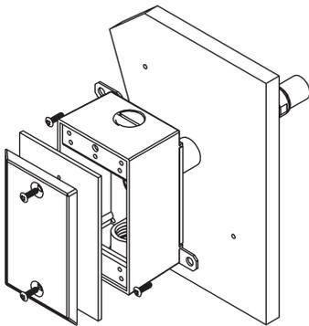
**Fig. 1:** Duct Humidity in a Weatherproof (WP) Enclosure
