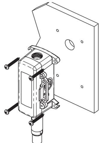
**Fig. 6:** Outside Humidity in a BAPI-Box 2 (BB2) Enclosure
