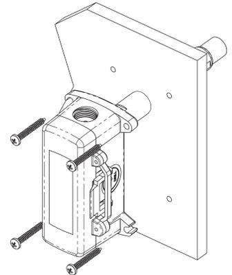
**Fig. 3:** Duct Humidity in a BAPI-Box 2 (BB2) Enclosure
