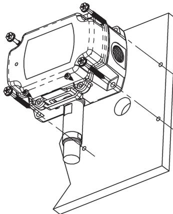
**Fig. 5:** Outside Humidity in a BAPI-Box (BB) Enclosure
