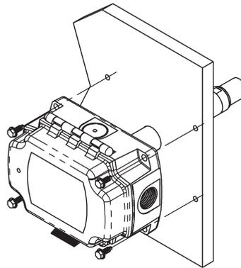
**Fig. 2:** Duct Humidity in a BAPI-Box (BB) Enclosure
