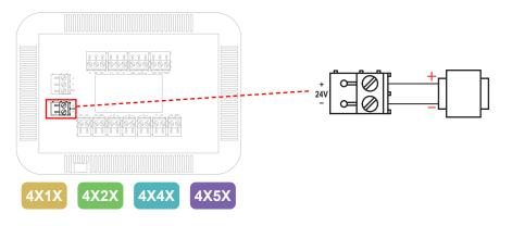
**Optional:** When used as a standalone thermostat with no communications, you can power the unit via the HVAC unit's transformer. To do this, install a jumper connecting the "R" and "+24" terminals. The "-24" terminal must then be connected to the common side of the unit transformer.
