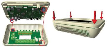
If it does not easily snap into place, check to make sure the internal connectors are properly aligned and reassemble the unit.
