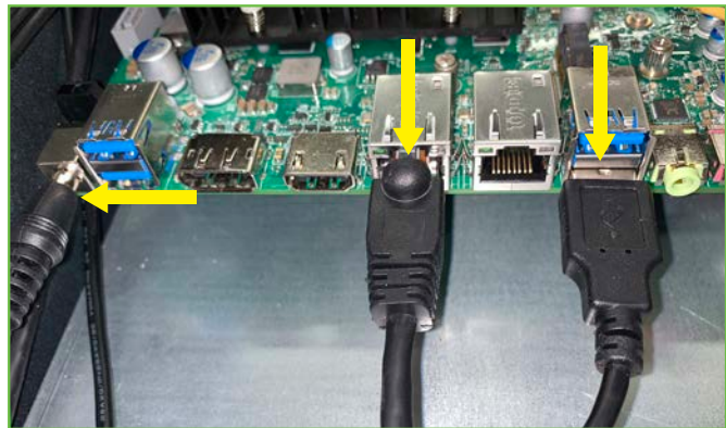
Closeup of Mother Board Power, USB, and Cloud Ethernet connections
