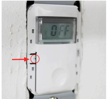
3. Press the Calibration button again. The words "Delay" will display. Delay sets the time-out period.
