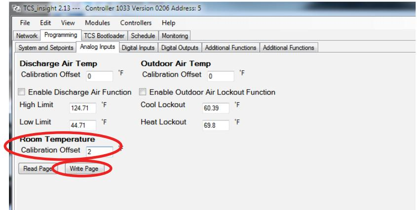
2. If the stat reads 74 degrees and the hand-held field device reads 72 degrees, type “-2” into the field and click “Write Page”.
