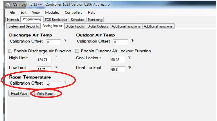
**E. Once calibration is completed, confirm temperature display on thermostat has changed, then disconnect QD1010 from thermostat.**
