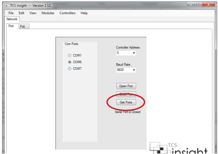
2. Select the proper 'Com Port' radio button and click the "Open Port" Button.
