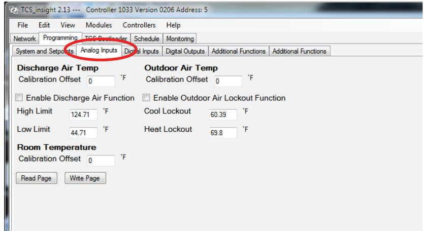
**D. Calibrate room temperature by changing Room Temperature Calibration Offset.**
