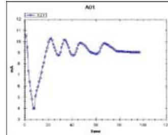
The graph still oscillates a little but ultimately settles down and does not continue to oscillate. Since the derivative factor is smaller it gets closer to the setpoint although it takes a little longer.
