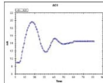
The oscillations settle down much quicker but the AO is slightly above setpoint although much closer to setpoints than the other graphs.
