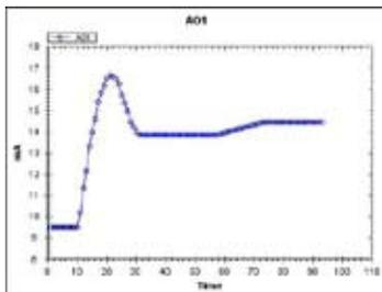
The graph levels off above the CFM setpoint because the Derivative factor is so high. The graph also does not oscillate very much to a step response, but is "over damped". Note the CFM graph tracks the AO1 graph almost exactly.
