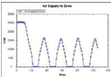
The graph continues to oscillate forever! An integral factor that is too large can cause oscillations, by increasing the PID delay it is possible to minimize the oscillations but they will still happen.
