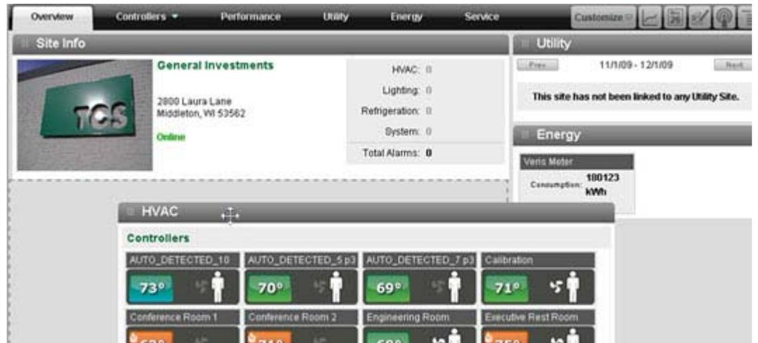
**Customize** -- In the upper right hand portion of the top tab bar, you will find a "Customize" button or a link. Clicking this button or link reveals a pop-up layer that allows you to hide or unhide various modules and tabs AND save any changes you made on that page (drag-n-drop sorting, starred sites, etc.).
