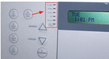
The LED lights indicate when the thermostat is in the occupied mode, and when the cooling, heating and fan are on. The LED lights for Service and Data are not enabled at this time.
