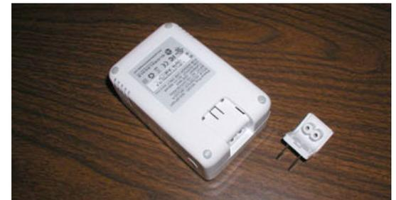
7. Plug the QD2010 into any "Surge"-only socket on the PK3100. DO NOT USE a socket which says "Surge/Battery" (If a PK3100 was not provided there is one already on site). The two lights on the QD2010 should flash and then come on solid. Once the lights are on solid for 10 minutes, contact TCS Technical Services to confirm the new QD2010 is contacting Ubiquity and the site is online. The QD2010 will show up in our system as an "orphan" until TCS Technical Services enters the QD2010's MAC address.
