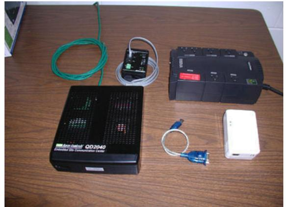
2. Remove the QD2010 and the PI1000 from their packages, and connect the PI1000 USB end to the QD2010 USB port.
