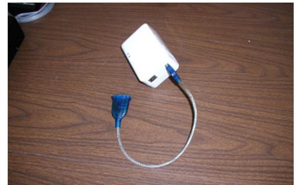
3. Disconnect the QD1010 cable and serial converter from the QD2040 and connect it to the serial end of the PI1000.
