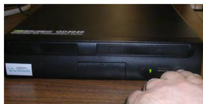
If the power LED is lit PLUS you are able to communicate locally AND to the Internet, run diagnostics on the QD/QWL device using the USB diagnostic tool (TCS Part Number PI4000).
