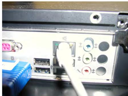
2. Determine the port that the device is plugged into and verify with your IT Department that this is the correct port.
