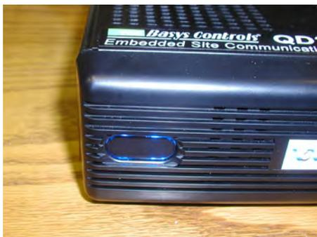
2. If not lit check the power cord on both ends to ensure it is plugged in tight and correctly to a working outlet, if plugged into a UPS (TCS Model PK3000 or PK3100) make sure that the UPS is powered on.
