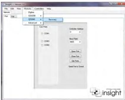
3. Select the QD Recovery Tab; enter in the MAC or Hardware Code for the device (this code can be found on a sticker on the back of the device), select the use code button, and select Action of: Run Diagnostics, click Save Action to USB.
