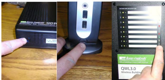
The QD2040-MAX has two buttons -- a reset and a power button. The reset button is the left button and the power button is the right button.
