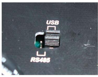
3. The RS485 mode is intended for the QW1010A to be used as part of a hardwired RS485 network, and is intended to be wired to a QD1010 via the RS485 terminal block.
