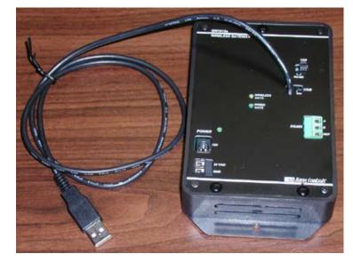
The USB mode is intended for the QW1010A to be used exclusively in a ZigBee wireless network and plugged directly into the USB port of the QD2040 or other computer.
