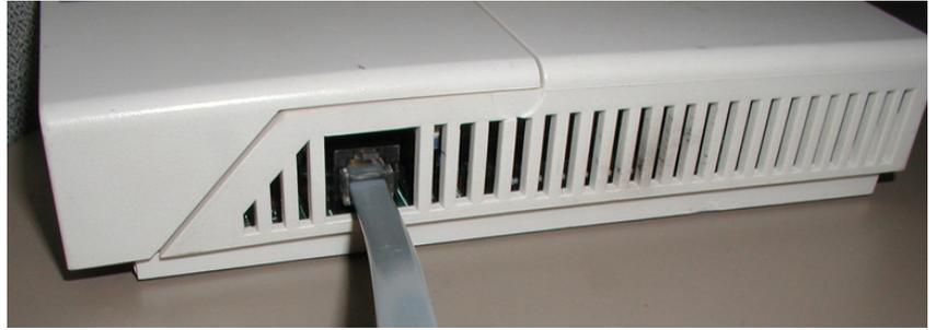
2. Plug the other end of the cord into the RS485 port on the QD1010-USB.
