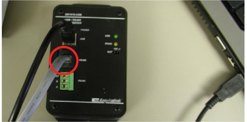
3. Insert the USB cable from the QD1010-USB to the USB Port on the laptop.
