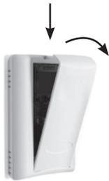
2. Remove the backplate by unfastening the sensor from the bottom of the backplate and pivoting the sensor outward.
