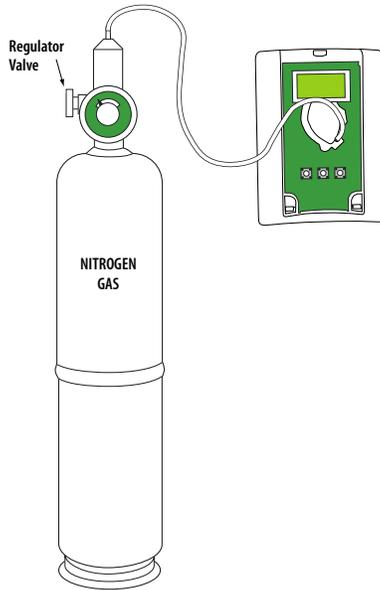
4. Calibrate for 5 minutes. Unit will return to run mode when calibration is complete.
