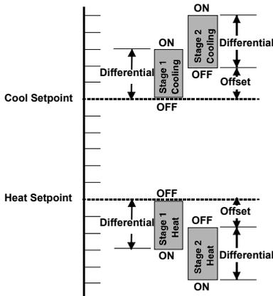
The SZW118 will control up to two stages of either heating or cooling.
