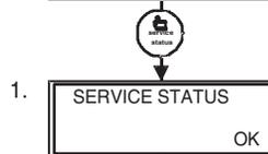
**Service Screen.** This message may be followed by any or all of the following: CHECK FILTER, CHECK FAN, DISCHARGE HIGH, DISCHARGE LOW, or CHECK DI2.
