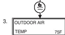
**Outdoor Air Temperature Screen.** Shows outdoor air temperature if sensor is used.
