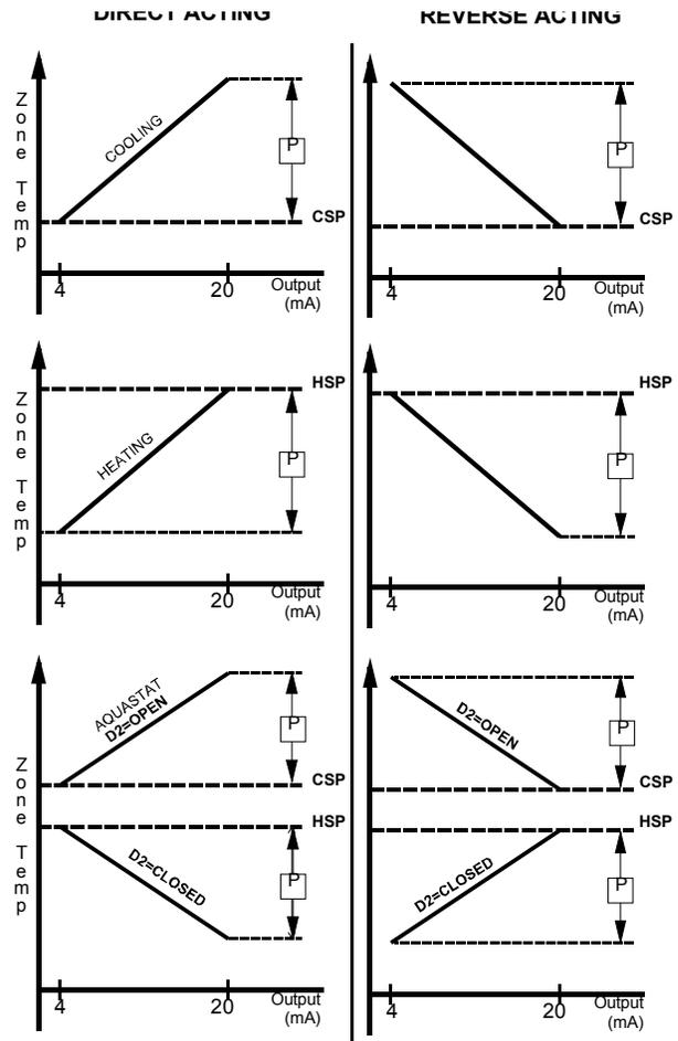
Select whether the analog output is set for heating, cooling or aquastat. Select direct or reverse action. Select whether you want the analog output to modulate from 4 to 20mA or 0 to 20mA. Select the unoccupied action ("20mA or 0 / 4mA" will hold the analog output device open or closed during unoccupied times. "Modulating" will modulate the analog output device to maintain the unoccupied heating or cooling setpoint.). Enter a proportional band (throttling range) in degrees.
