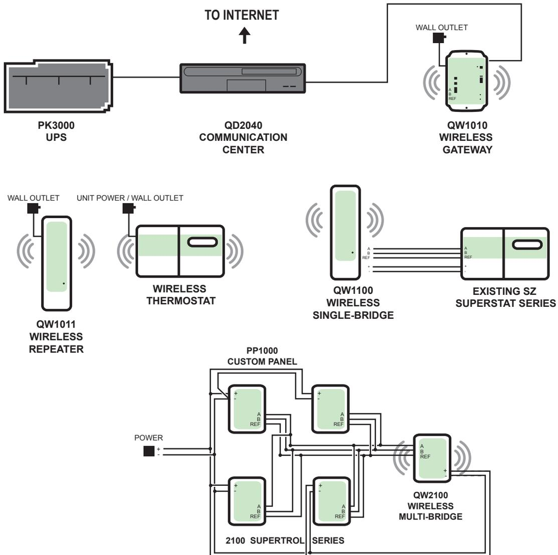
**NOTE:** max distance for indoor ZigBee wireless network is 150' to 500' depending on conditions.
