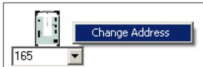
default address for an SL2105 is 105 and the default address for an SL2108 is 108. You can either type in the address, or choose the particular controller by location. For controllers with multiple initialization screens, the address of the controller is only entered on the first screen. To modify the address, click Change, enter the new address in the window and then click OK. If the address shown in screen A updates to the new address, the change has been completed.
