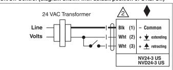
On/Off Control-using actuator to drive one direction and spring the opposite direction. NOTE: A bridge must be made inside the NVF between terminals 2 and 3 (diagram shown with default position of S3.2: 3-way Off, 2-way On)
