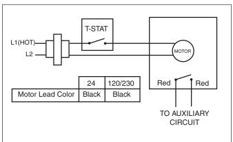
Built-in Auxiliary Switch (optional) (-S models)
