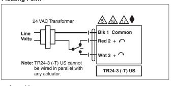
Refer to page 26 for auxiliary switch (-S models) and -P5, -P10 potentiometer wiring.
