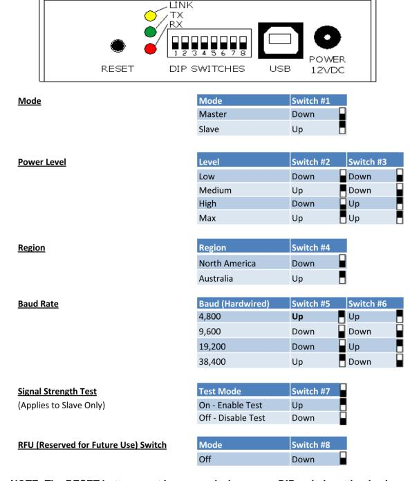
NOTE: The RESET button must be pressed whenever a DIP switch setting is changed.
