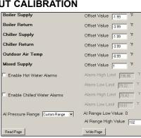
that the actual input temperature has been adjusted. For example: You measure the hot water supply temperature and it reads 71°. The SZ2165 reading is 72° and the Hot Water Supply Temperature already has an offset of -2.0°. All you need to do is change the offset value to -3.0° and you're done. The SZ2165 will now read 71°.
