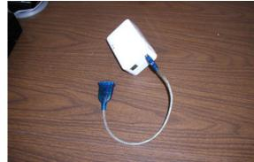
NOTE - The USB port on the QD2010 is fairly shallow. Even when fully inserted into the port, the plug may appear to have 3/16" left to insert. DO NOT force the plug past its normal stopping point. DOING SO WILL DAMAGE THE UNIT and WILL VOID the QD2010's warranty.
