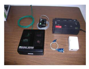
2. Remove the QD2010 and the PI1000 from their packages, and connect the PI1000 USB end to the QD2010 USB port.
